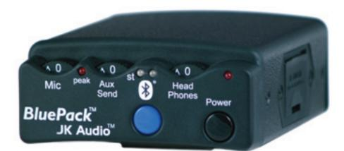
plenty of power available – and the usual warnings and disclaimers are made regarding high listening volumes in the compact manual. There are also four LEDs: one each for peak levels on the mic and line inputs, one for Bluetooth indications and one to show when the unit is powered.
