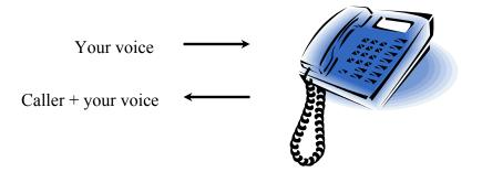
The presence of your voice on the handset receiver is known as "Sidetone". This audio path gives the user immediate feedback, letting them know that they are speaking into the handset at an appropriate level. Simple recording taps will not allow you to adjust the level of your
