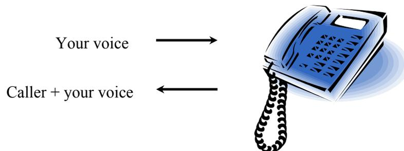
The presence of your voice on the handset receiver is known as “Sidetone”. This audio path gives the user immediate feedback, letting them know that they are speaking into the handset at an appropriate level. Simple recording taps will not allow you to adjust the level of your
